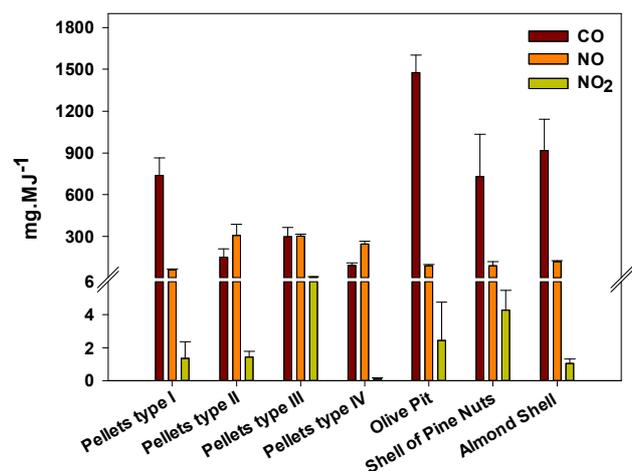
Figure 1. CO, NO and NO<sub>2</sub> emission factors for the combustion of different fuels (mg MJ<sup>-1</sup>).
