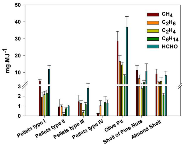
Figure 3. CH<sub>4</sub>, C<sub>2</sub>H<sub>6</sub>, C<sub>2</sub>H<sub>4</sub>, C<sub>6</sub>H<sub>14</sub> and CHOH emission
