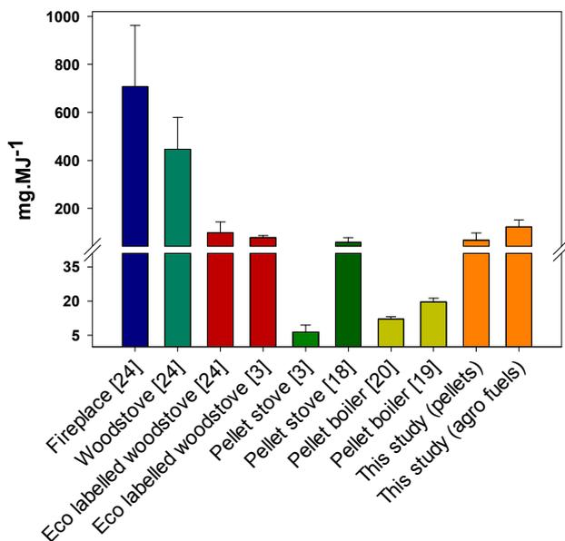
Figure 4. Particulate matter emissions from different types of small-scale combustion appliances ( $mg MJ^{-1}$ ).
