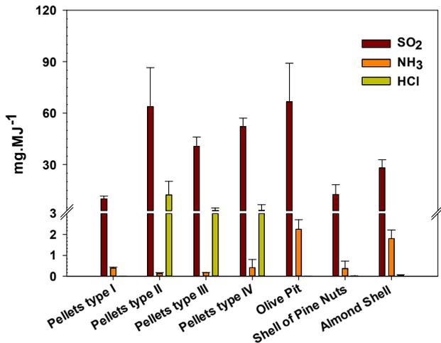
Figure 2. SO<sub>2</sub>, NH<sub>3</sub> and HCl emission factors for the combustion of different fuels (mg MJ<sup>-1</sup>).
